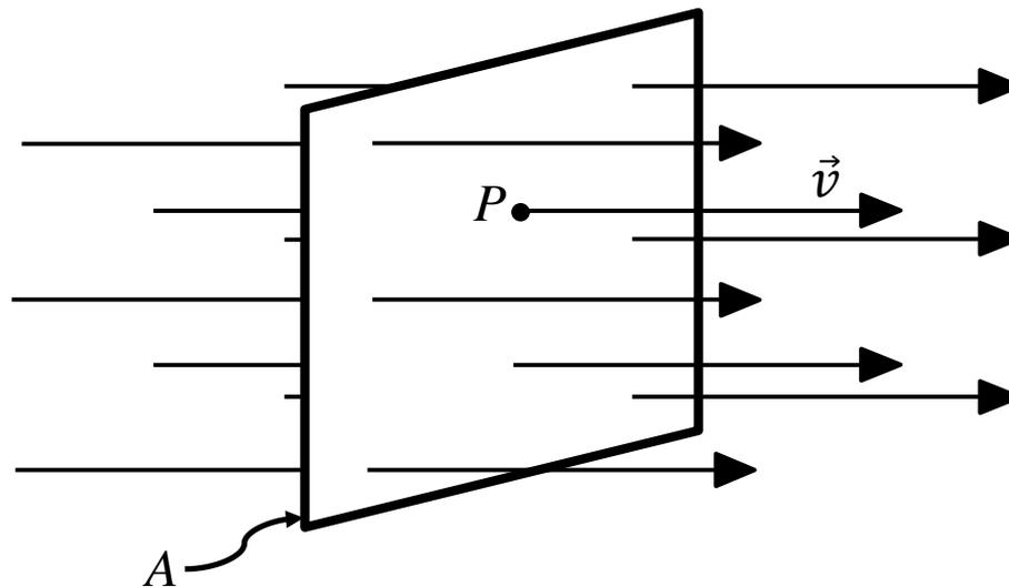
Let  $\Phi$  represent the “volume flow rate” through the loop. That is,
