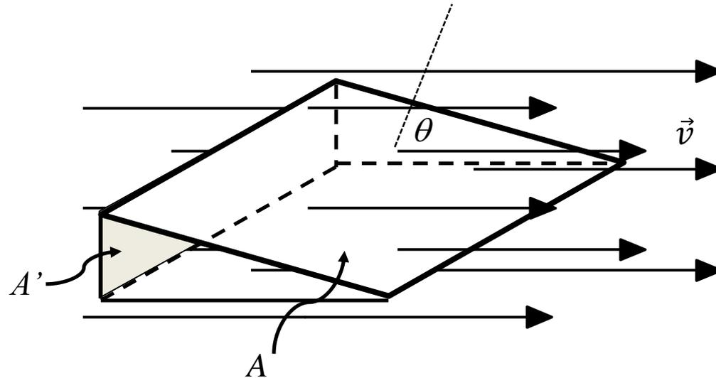
Since the volume flow rate depends on the component of  $\mathbf{v}$  that is normal ( $\perp$ ) to the plane of the loop ( $v \cos \theta$ ) we can write the flow rate or **volume flux** (in this example) as
