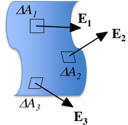
In this case, the electric flux through the surface by summing over all the  $\Delta A$ 's where each  $\Delta A$  is small enough to consider the  $\mathbf{E}$ -field through that  $\Delta A$  to be constant. Then,
